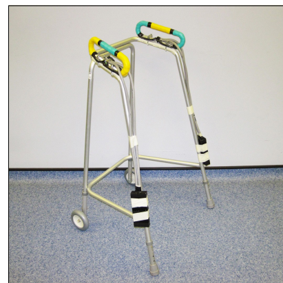
Figure 1. Instrumented handles fixed on an anterior walker
